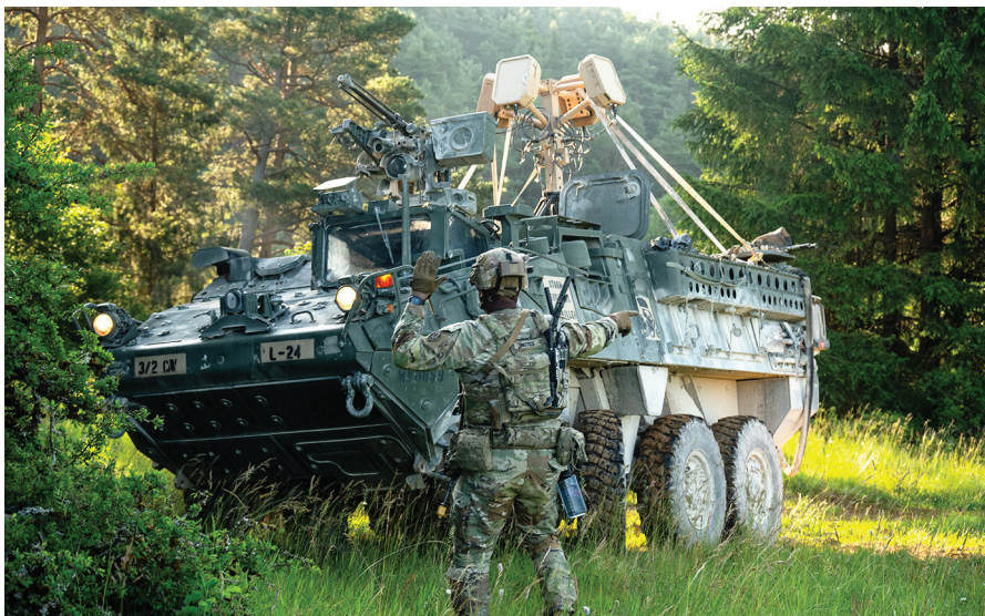
A soldier with the 2nd Cavalry Regiment guides a Stryker mounted with an EchoShield cognitive radar into concealment June 20 during Project Flytrap, a series of counter-unmanned aerial system exercises, in Hohenfels, Germany. (U.S. ARMY/SPC. ELIJAH MAGANA)
